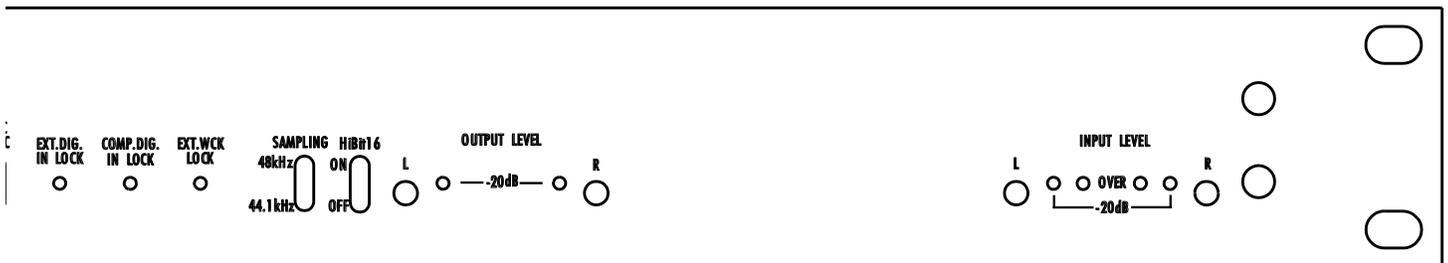
Sets the sampling of the ADC and control bits on all digital outs. Must be always set right for digital transfers.
